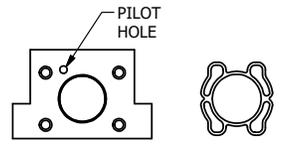
ALIGN PILOT AND SLOT IN ADAPTOR WITH GASKET IN BETWEEN, BOTH SIDES. FOR EXTERNAL PILOT OPERATION - ROTATE ADAPTOR 180 DEGREES. REMOVE 1/8" NPTF PLUG AND SUPPLY 50-150 PSI TO 1/8" NPTF PILOT PORT IN ADAPTOR.
