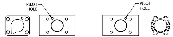
POSITION GASKET ON END OF VALVE TO SEAL PILOT HOLE SIDE 'B' ONLY
