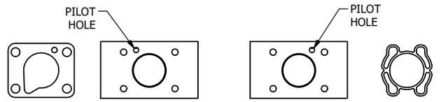
POSITION GASKET ON END OF VALVE TO SEAL PILOT HOLE SIDE 'B' ONLY
