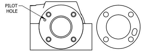
POSITION GASKET TO SEAL PILOT HOLE, BOTH SIDES.
