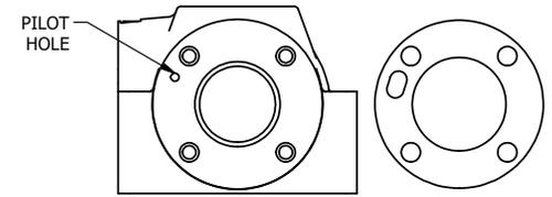
ALIGN PILOT AND HOLE IN GASKET, BOTH SIDES.
