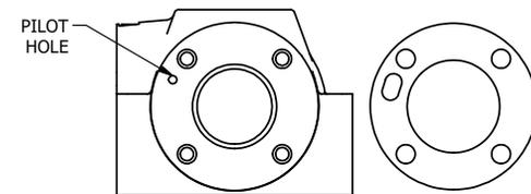
ALIGN PILOT AND HOLE IN GASKET, BOTH SIDES.
