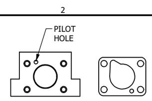
ALIGN PILOT HOLE AND CENTER CUTOUT ON BOTH SIDES.
