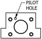
ALIGN PILOT HOLE AND CENTER CUTOUT ON BOTH SIDES.
