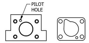
ALIGN PILOT HOLE AND CENTER CUTOUT ON BOTH SIDES.
