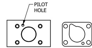
ALIGN PILOT HOLE AND CENTER CUTOUT ON BOTH SIDES.
