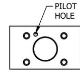
ALIGN PILOT HOLE AND CENTER CUTOUT ON BOTH SIDES.
