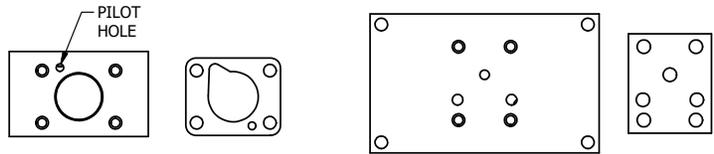
ALIGN PILOT HOLE AND CENTER CUTOUT ON BOTH SIDES.
