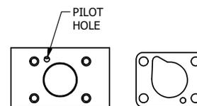
ALIGN PILOT HOLE AND CENTER CUTOUT ON BOTH SIDES.
