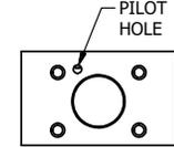
ALIGN PILOT HOLE AND CENTER CUTOUT ON BOTH SIDES.
