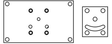
ALIGN HOLES IN GASKET AS SHOWN. FOR EXTERNAL PILOT PRESSURE, REMOVE PIGGY BACK BLOCK AND ROTATE 180°. LEAVE GASKET AS SHOWN. REMOVE 1/8" PLUG AND CONNECT SUPPLY PRESSURE - 160 PSI MAX.
