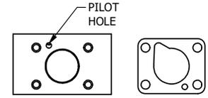
ALIGN PILOT HOLE AND CENTER CUTOUT ON SIDE 'A' AS SHOWN.
