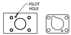
ALIGN PILOT HOLE AND CENTER CUTOUT ON SIDE 'A' AS SHOWN.
